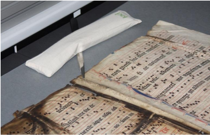
Pellet weight and metal spatulas used for support in scanning.
